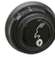
KEY LOCKING FRONT READ DIAL Key is used to lock dial in a fixed position and affords dual custody control. Manager has the combination, collector has the key. Both must be present to unlock the safe.
